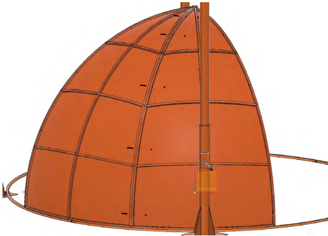
Figure 35. Align adjacent carpels' five bolt holes.
