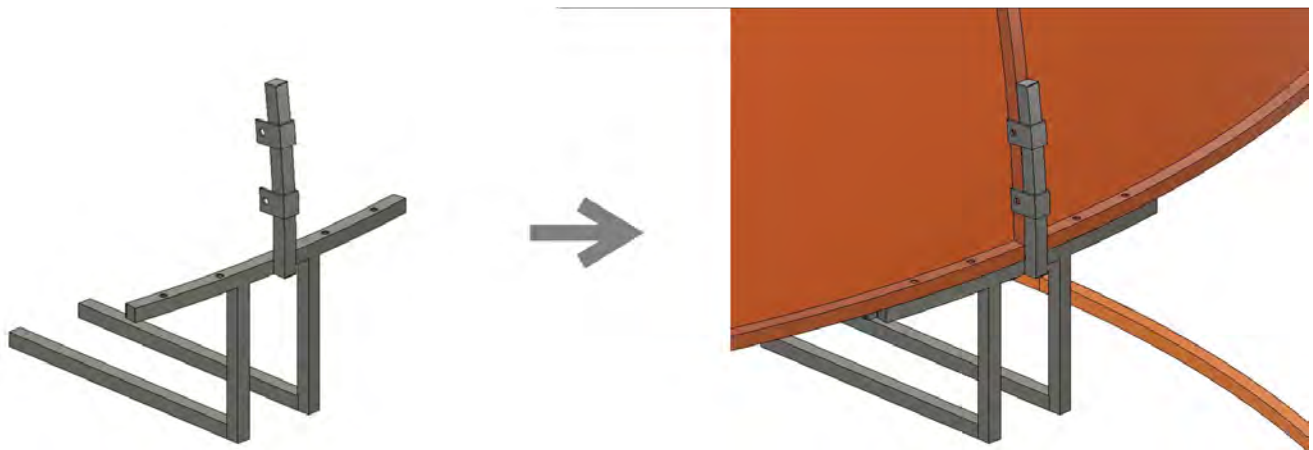
Figure 40. Align the holes on the outer holder with the holes on the projection carpel's supports.
