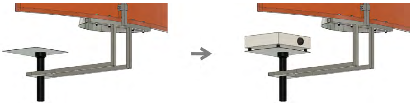
Figure 44. Place the projector atop the plate and secure.
