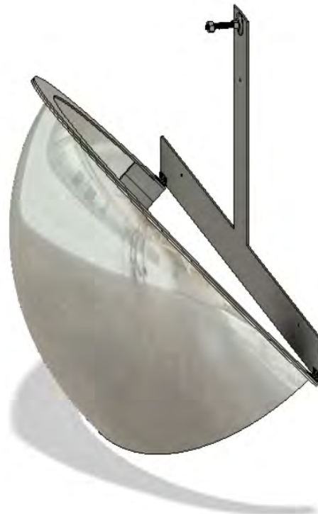
Figure 16. The mirror system consists of a T-shaped steel plate and a curved mirror holder joined together with hinges. The mirror is riveted to the holder, so the mirror system comes as a singular component.
