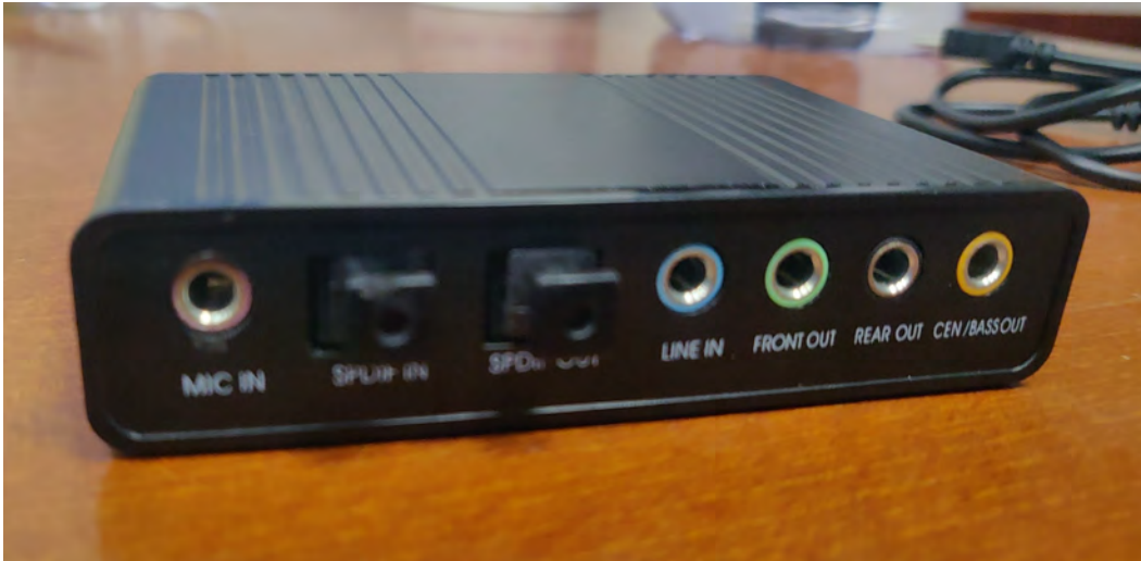
Figure 22. A 5.1 channel sound card with 3 × 3.5 mm audio output jacks.
