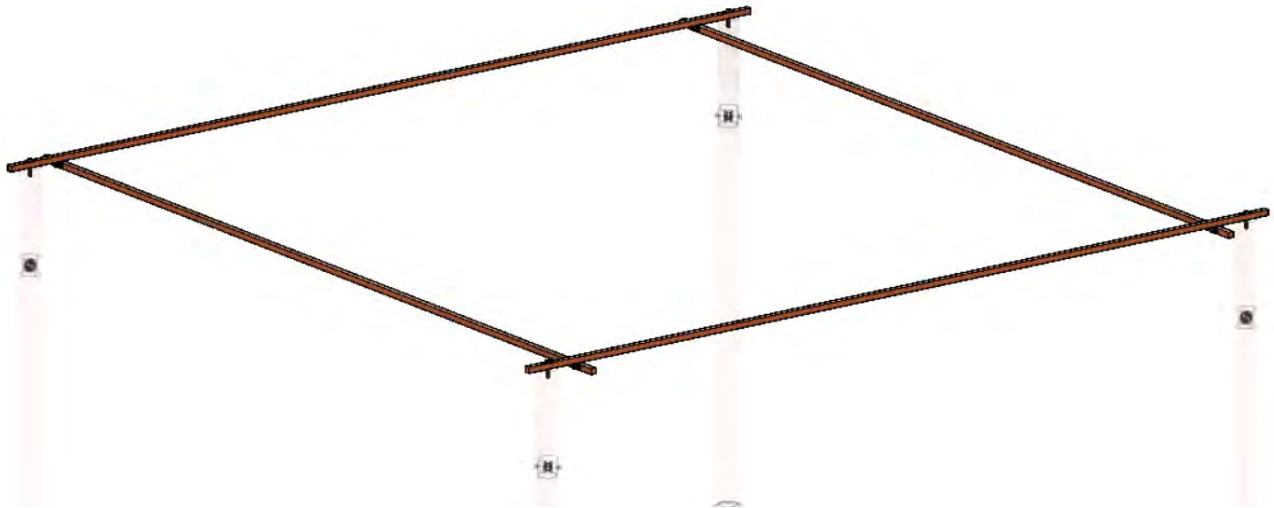
Figure 12. The top supports securing the (translucent) poles.
