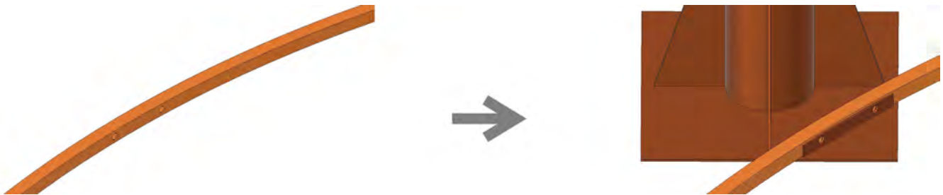
Figure 26. How the pole should be positioned with respect to the ring.
