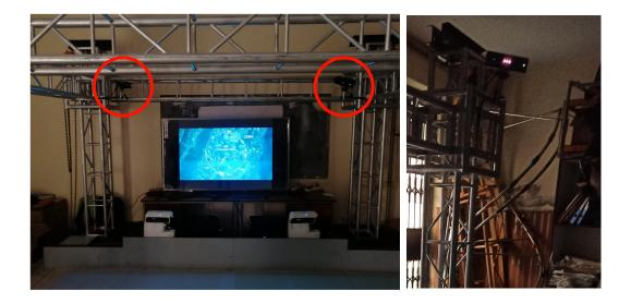
• Tighten the screws of the short-throw projectors mounts and attach the projectors on it. Roughly align the projectors or we can do the alignment part when aligning the displays.
