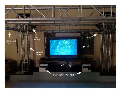
• After all parts of the truss gets unloaded, place the four vertical truss in the four dollies. Next, align the horizontal columns with the dolly such that two 6 feet horizontal columns are on the sides of the structure whereas the other two 10 feet horizontal columns are on the front and back. Align the ends with dolly and screw them up.
